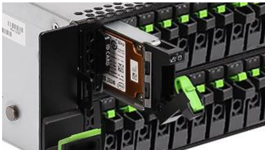
Figure 1: E1 SSDs in a dense 2U rack unit
